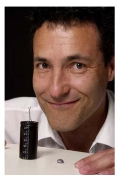
Mike Cortie shows two capacitors. The big one is made by conventional technology and the small one has the same capacitance but is made using mesoprous gold (a sponge made of gold nanoparticles)
