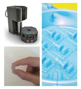
Figure 10: An NV diamond chip-set that is optically coupled, placed inside a 4K helium cryostat system.
