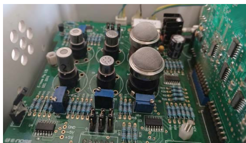
Figure 1: Mark 4 E-Nose by Enose Pty Ltd showing six sensors. (Photo G Bell).
