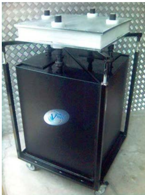
Fig 5: V-Fuel integrated battery on a trolley, with pumps and piping incorporated inside tanks.
