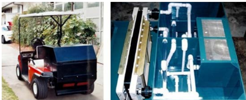
Fig 3: VFB powered electric golf cart at UNSW in 1997 (Left). Compact stack and tanks with hidden plumbing designed for the golf cart (Right). Photos courtesy Maria Skylas-Kazacos UNSW Sydney.
