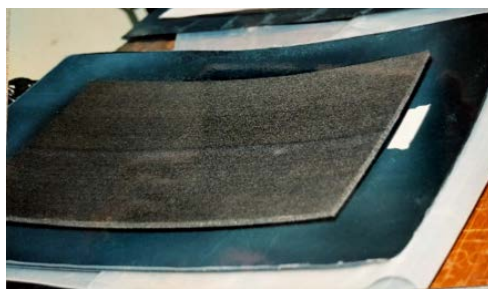
Fig 1: Bipolar electrode fabricated by heat bonding graphite felt sheets onto each side of the conducting plastic sheets developed by UNSW.
