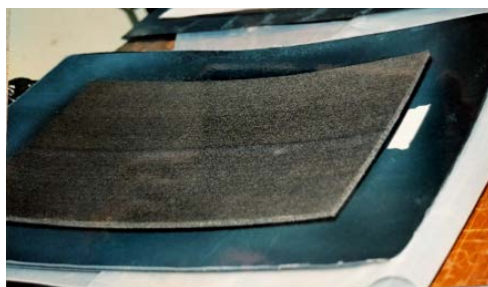
Fig 1: Bipolar electrode fabricated by heat bonding graphite felt sheets onto each side of the conducting plastic sheets developed by UNSW.
