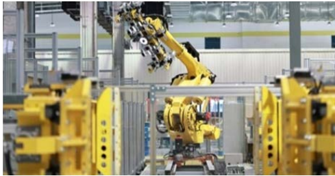
Fig 7: Automated stack assembly at Rongke Power, China (reproduced with permission of Rongke Power).
